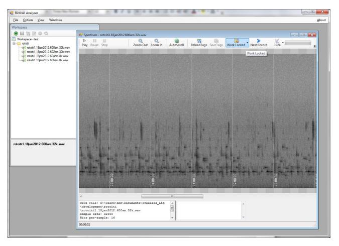
On the spectrogram toolbar, note the 'Work Locked' tag. This prevents changes to the analysis, until you are ready to start work.
